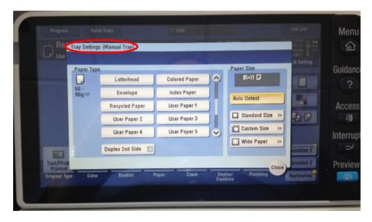
The other thing is that the paper settings for the bypass tray will need to be set for "index paper". Once this is set up and the tabs are set up your ready to print.
