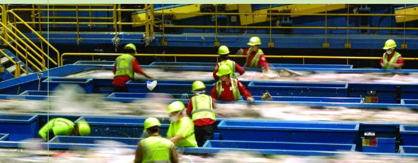
*The Elkrige MRF uses a combination of manual and mechanical technologies to separate the mixed recyclables that arrive at the facility in a "single stream."*
